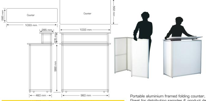
MATERIAL: Silver color (anodised) aluminium & 18 mm thick laminate hardboard COUNTER SIZE (Y\*X) SIDE PANELS ITEM CODE FRONT PANEL 846 x 476 mm 846 x 285 mm 1033 x 562 mm Pano D2-DZ70 760 x 956 mm 360 x 956 mm Upper Block Pano D2-DZ90 760 x 187 mm 187 x 187 mm 960 x 956 mm 460 x 956 mm Upper Block 1033 x 285 mm 960 x 187 mm 187 x 187 mm Portable aluminium framed folding counter.
