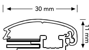
**EXTRUSION: SILVER COLOR (ANODIZED) ALUMINIUM****FRAME PROFILE: 30 mm**
