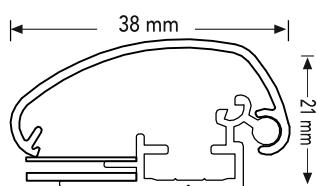
**EXTRUSION: SILVER COLOR (ANODIZED) ALUMINUM****FRAME PROFILE: 38 mm**
