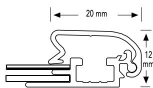
**EXTRUSION: SILVER COLOR (ANODIZED) ALUMINIUM****FRAME PROFILE: 20 mm**
