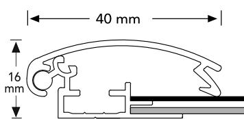
**EXTRUSION: SILVER COLOR (ANODIZED) ALUMINUM****FRAME PROFILE: 40 mm**
