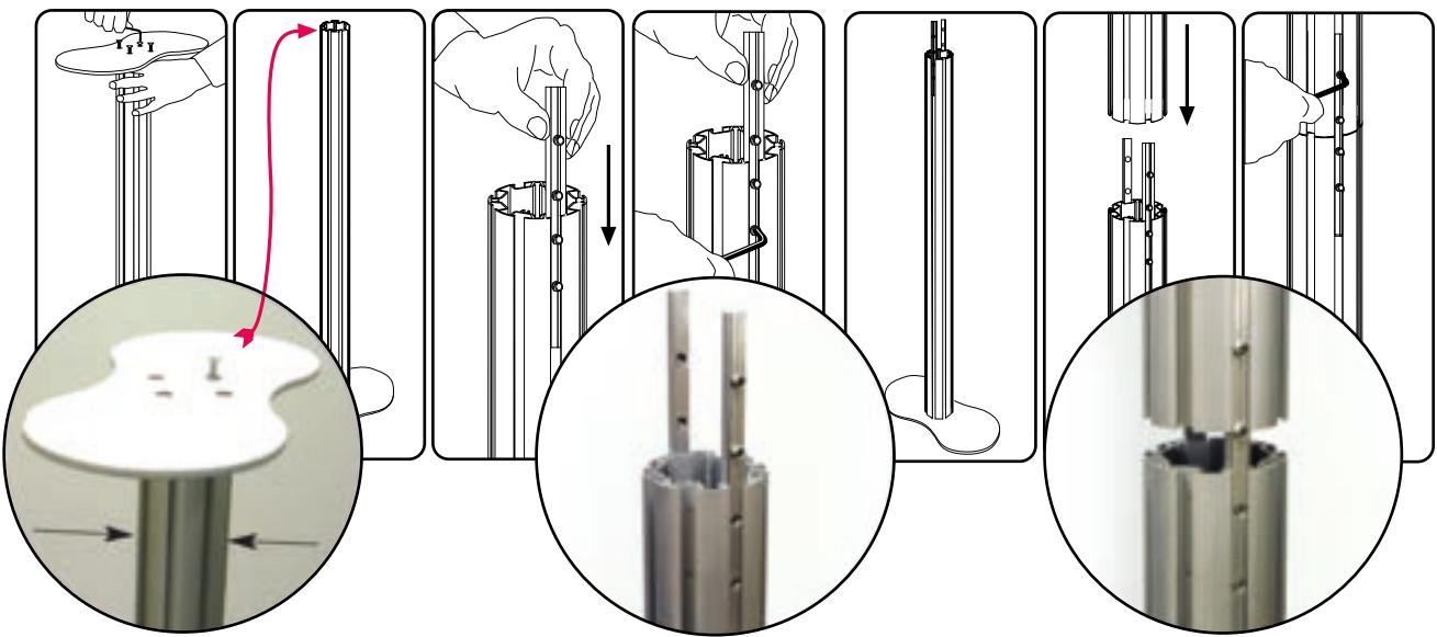
Attach base plate to lower column.
